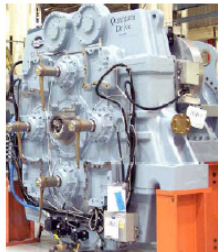
Fig. 5 Clipper Quantum Drive, gearbox architecture [8], [9]
